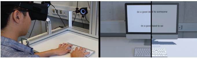
Preliminary work by project C06: Example of a Mixed Reality workspace enabling gradual blending between a physical and virtual environments
